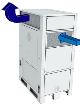
Figure 4: Air intakes and outtakes
