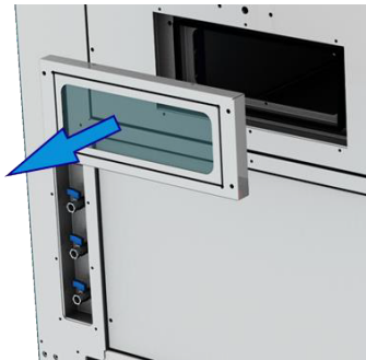
Figure 24: Condensation tray access panel
